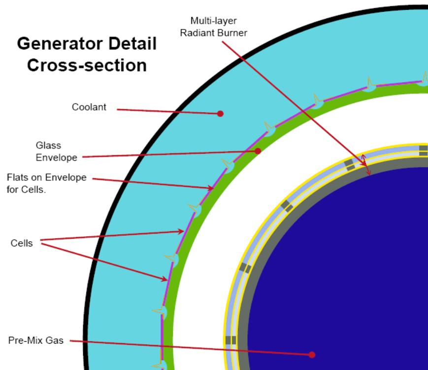
**FIGURE 2.** The IR cell array is bonded onto a glass cylinder and cooled from its backside. There is an IR filter coating on the outer surface of the glass cylinder that reflects mid-wavelength radiation back to the SiC fibrous emitter.
