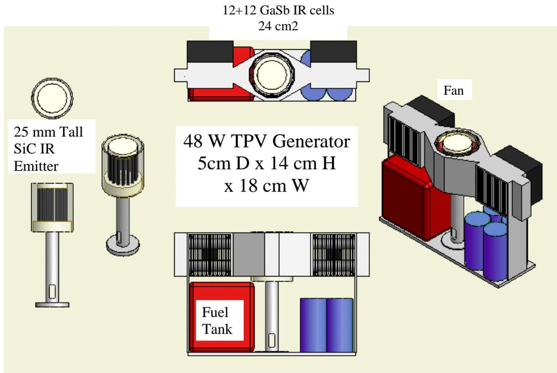
**FIGURE 3:** Compact and powerful TPV demonstrator using boiling liquid cooling built around a Bunsen burner.
