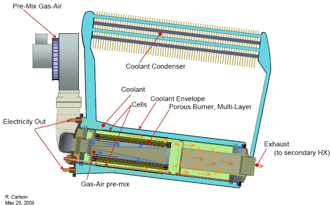
**FIGURE 1.** Cross section of Simplified Cylindrical TPV Generator showing flow through SiC emitter surrounded by an IR cell array immersed in a boiling coolant. The coolant condenses in an air heat exchanger and is returned to the TPV generator by gravity.
