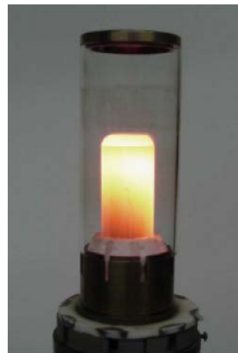
Figure 21: AR coated Pt IR emitter test.
