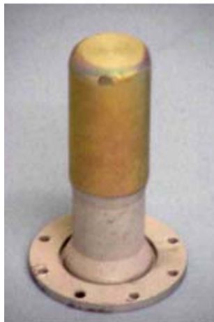
Figure 20: AR coated W IR emitter (radiator).
