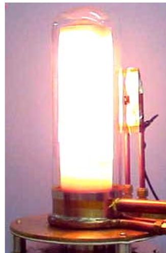
FIGURE 6. The power output of a single GaSb cell was measured in combination with a radiant tube burner and an emitter thermos as shown in the photograph on the right. The results tabulated on the left suggest that a system electrical conversion efficiency of 16% should be achievable with a complete system.
