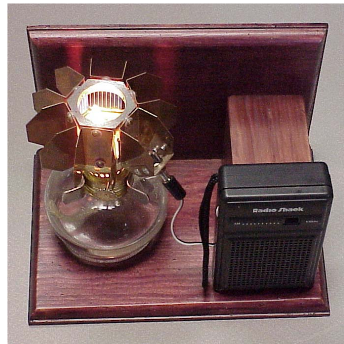
Oil Lamp with TPV cylinder operates radio
